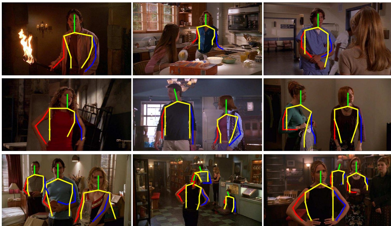
Fig. 13: Results on the Buffy dataset. We visualize all skeletons (instead of boxes) reported by our algorithm for a given image, after non-maximum suppression (NMS). Our model hence serves as both an articulated detector and pose estimation algorithm, as evidenced by our average-precision of keypoints (APK) measure.
