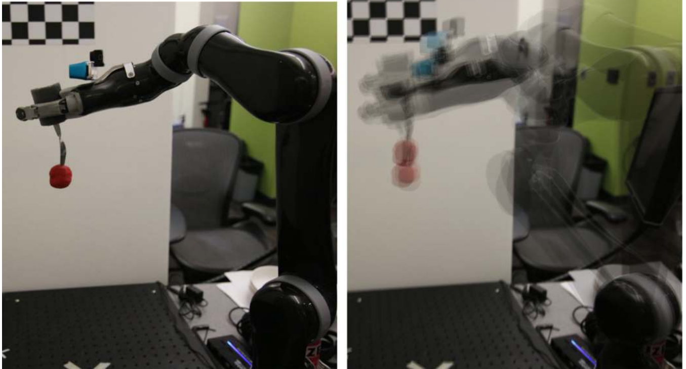
Fig. 2. The Kinova Mico robot was sent to 10 inverse kinematics solutions for a fixed pose (left). The solutions are overlaid on the right. Error at the end effector exceeds 5 cm.
