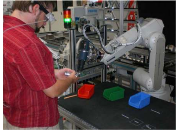
Fig. 20. Picture of a worker wearing eye-tracking glasses and fixing screws together with the robot on a product in the hybrid assembly cell (CoTeSys/Kurt Fuchs).
