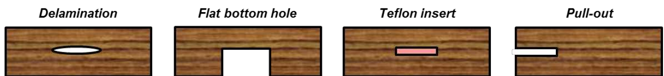
Figure 1. True delamination and 3 methods of artificial defects in CFRP laminates for UT NDI.
