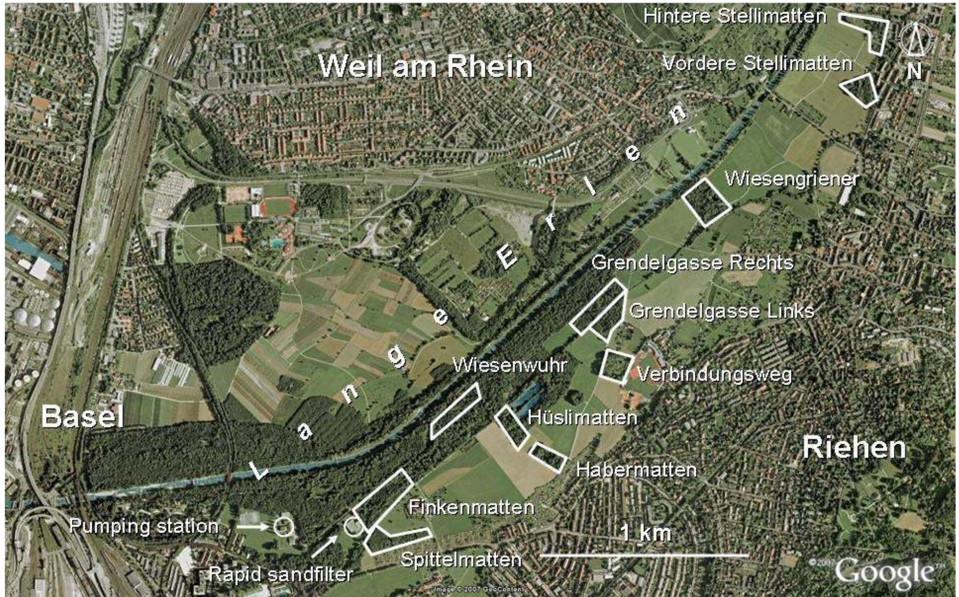
Fig. 1: The study site "Lange Erlen", Basel (Switzerland). Framed areas represent the current recharge areas (status 2008).
