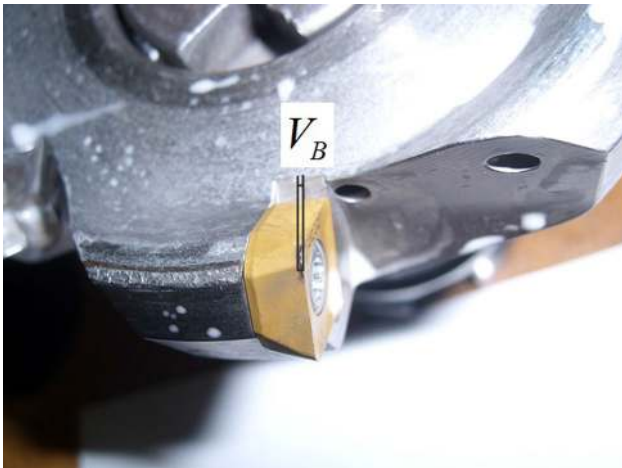
Fig. 1 Wear of changeable indexable insert (CII) on the plowing surface: flank wear V_B
