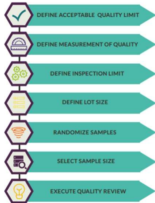
Fig. 6 Defining acceptable quality limit (AQL) parameters. The step by step process of defining AQL parameters, in order to perform quality review
