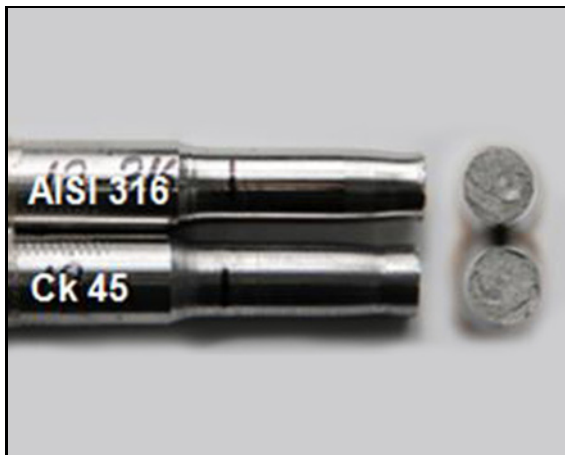
Fig. 3. Macroscopic view of the tensile test.
