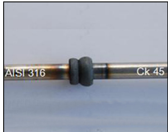
Fig. 2. Macroscopic view of the welded specimen.
