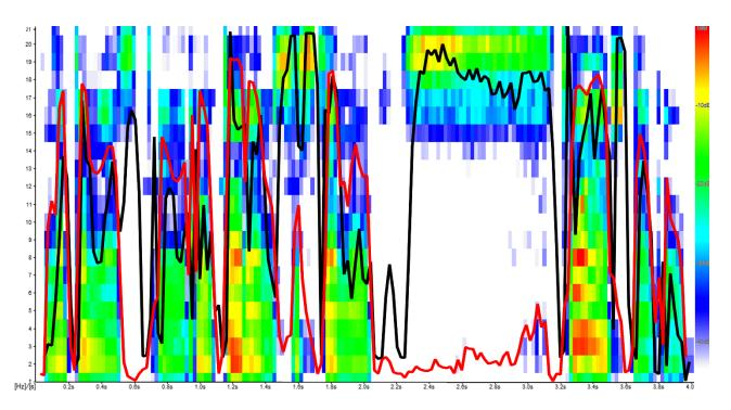
**Figure 5.** Prolongation spectrogram with  $G_1$  (red) and  $G_2$  (black) components. As can be observed, the shape of both G1 and G2 reflects the general time-frequency structure of the analysed utterance, but it is G2 which reflects higher frequencies while G1 concentrates on the lower ones instead.
