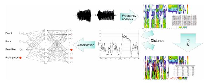
**Figure 1.** The experiment outline. The speech signal is transformed with FFT, 1/3 octave filters, and A-filter. Next, the PCA algorithm is applied. Based on the PCA model, the distances between new (PCA) and previous system of coordinates are calculated, and then the classification process with multilayer perceptron is conducted.
