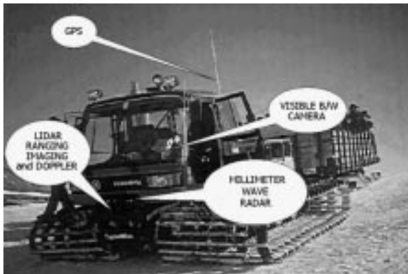
Fig. 5. Sensing capabilities of the platoon leading vehicle.
