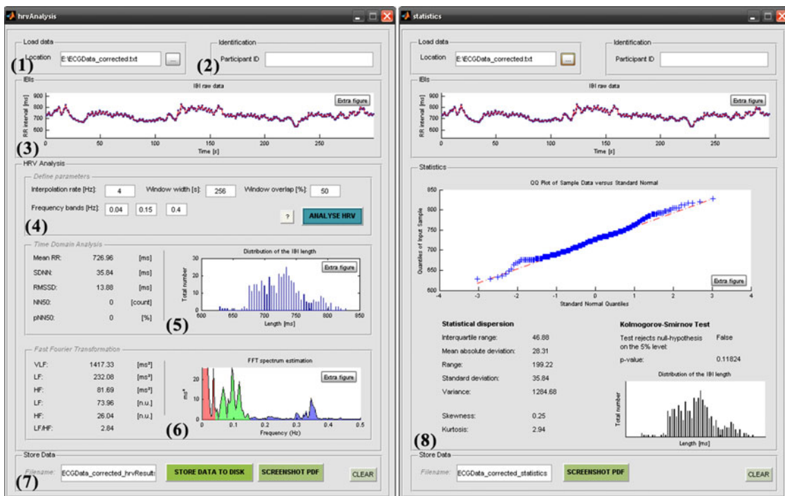
Fig. 4 The graphical user interface of hrvAnalysis and descriptiveStatistics. 1 Load data. 2 Insert participant ID (optional). 3 Raw data plot. 4 Settings for HRV computation. 5 Time domain analysis. 6 Frequency domain analysis. 7 Store data. 8 Distribution statistics
