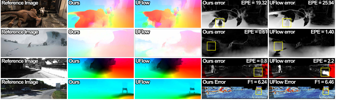
Figure 6. We show qualitative comparisons with the state-of-the-art method UFlow [14] on online evaluation benchmarks, including Sintel Clean (first row), Final (second row), KITTI 2012 (third row) and 2015 (last row). The error maps of predictions are visualized in the last two columns. In error maps, brighter regions indicate the larger estimation errors except that visualized by KITTI 2015 benchmark where correct estimations are displayed in blue and wrong ones in red.
