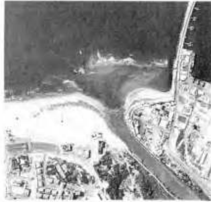
Figure 12. Aerial photograph taken on 14 February 1992, 10 days after the flooding of Lakhish River, showing the shoal which was formed in front of the river's mouth.
