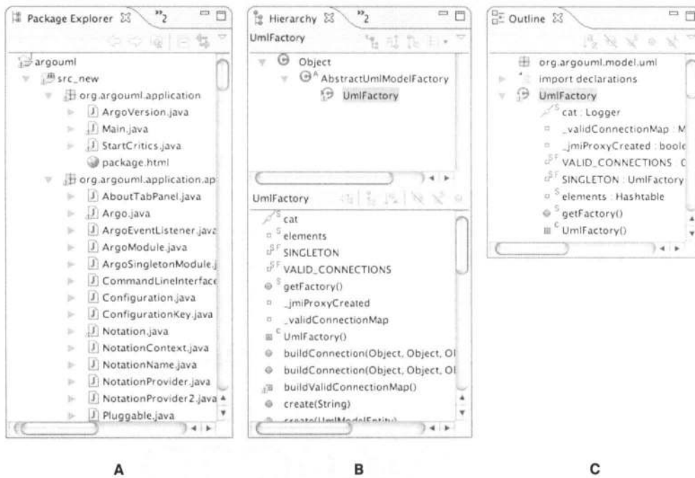
Figure 6.1: Three tools provided as part of the Eclipse Java Development Environment: (A) the Package Explorer which shows the package, file and class structure of a code base, (B) the Type Hierarchy which shows portions of a code base's inheritance structure, and (C) the Outline View which provides an overview of the contents of a particular source file.
