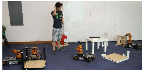
Figure 1: A robot engaged in assembling an IKEA LACK table requests help using natural language. A vague request such as “Help me” is challenging for a person to understand. Instead, this paper presents an approach for generating targeted requests such as “Please hand me the black table leg.”
