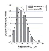
Figure 5. Quantitative distribution function of diffusion bridges between fibers
