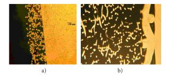
Figure 3. Porous structure with the base: a – fibrous; b – reinforced copper mesh
