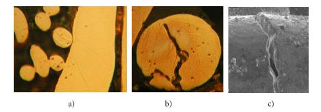
Figure 8. The effect of "hydrogen disease": in structure (a) in the fiber (b) and the copper mesh (c)
