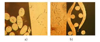
Figure 6. The fragment of the fiber contact with the base (a) and the base with the mesh (b) in the copper structure
