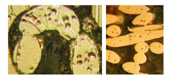
a) b) Figure 10. The effect of "hydrogen disease" on copper fiber bridges (a, b)
