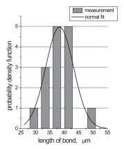
Figure 9. Quantitative distribution function of diffusion bridges between the copper surface and randomly spun fibrils (diameter of mesh bridges with copper substrate)
