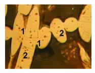
Figure 4. Diffuse fusion of fibers on the grain boundary (1) with pores (2)
