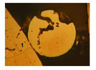
Figure 7. Effects of "hydrogen disease": open (2) and closed (3) pores on fibers and grain boundaries (1)
