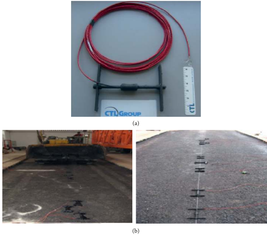
FIGURE 8: Asphalt strain sensor model ASG-152: (a) photograph and dimension of ASG-152; (b) ASG-152 layout.
