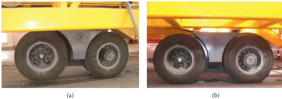
FIGURE 11: Loading modes: (a) single-axle loading mode; (b) dual-axle loading mode.
