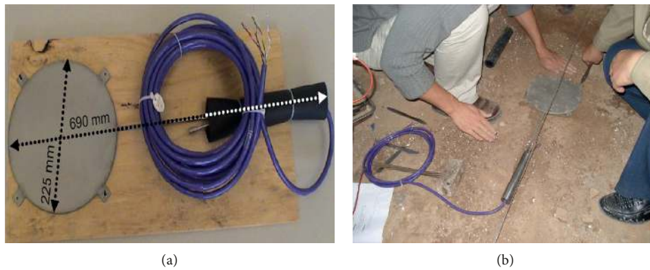
FIGURE 9: Pressure cell model Geokon-3500: (a) photograph of Geokon-3500; (b) Geokon-3500 layout.
