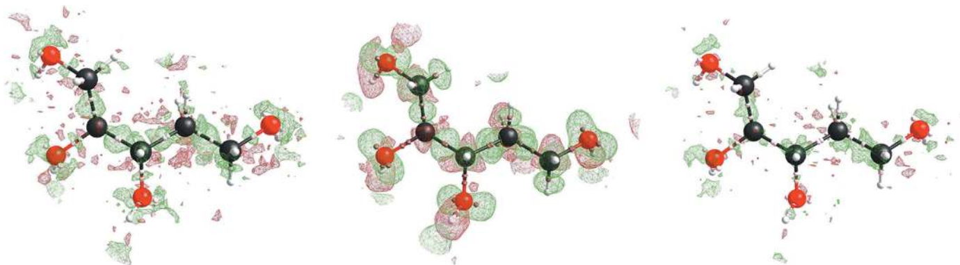
Figure 3 Left: xylitol (sh5011) residual IAM density at ISO level 0.1 e Å -3 . Center: BODD deformation density added to the IAM. Right: remaining residual density after adding the BODD deformations. IAM \Delta\rho_{\max}/\Delta\rho_{\min} = 0.33/-0.20 ; BODD \Delta\rho_{\max}/\Delta\rho_{\min} = 0.23/-0.22 .
