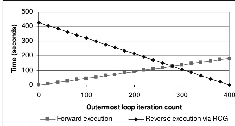
Figure 34: The elapsed forward/reverse execution times versus various program points in 400x400 matrix multiply.
