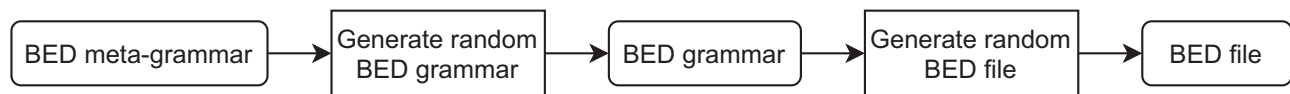
Fig. 3. Flowchart depicting grammar-based fuzzing. Rounded rectangles: files; sharp rectangles: generators. The BED meta-grammar describes different BED grammars to introduce further variation in the generated BED file
