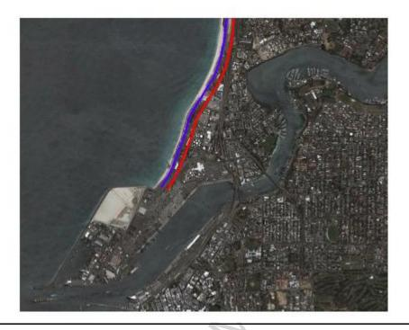
Figure 4. SMIC Model predicted coastline change at Swan River inlet, Australia by 2100 (red line) and coastline change due to the Bruun effect alone (blue line) (after Ranasinghe et al., 2013).
