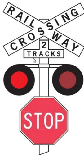
Figure 4: Symbolic representation of the visual human machine interface – Train approaching case.
