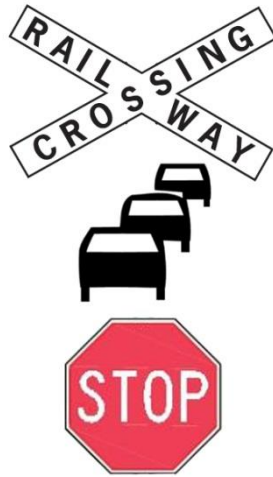
Figure 5: Symbolic representation of the visual human machine interface – Congestion case (The vehicles are flashing in red)
