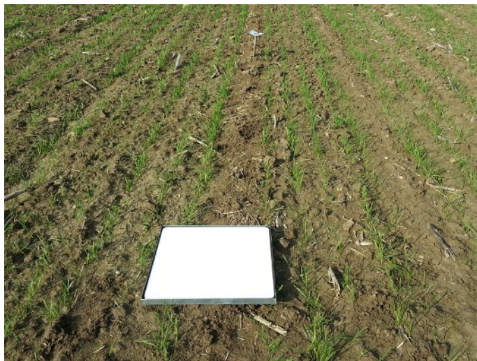
Figure 3. Details of experiment setup to assess spectral discrimination: Spectralon panel placed in the middle of the study area.
