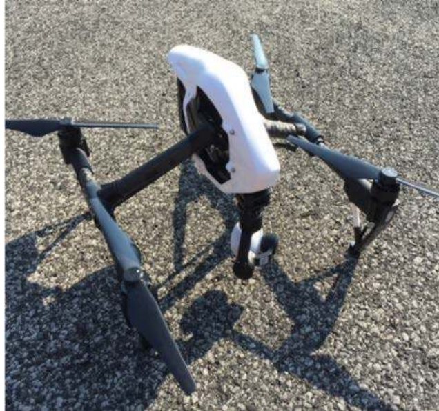
Figure 3.4 UAS used in the study, DJI Inspire 1
