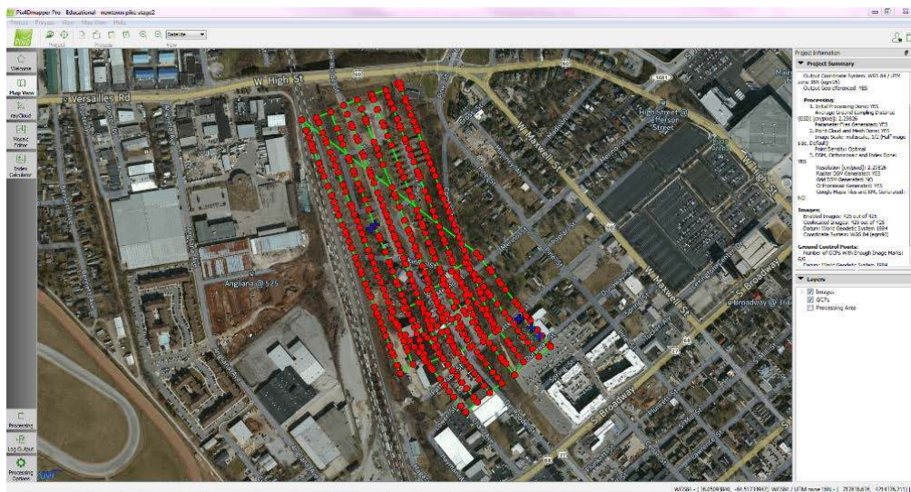
Figure 2.4 Grid Mission Plan for Stage 2.
