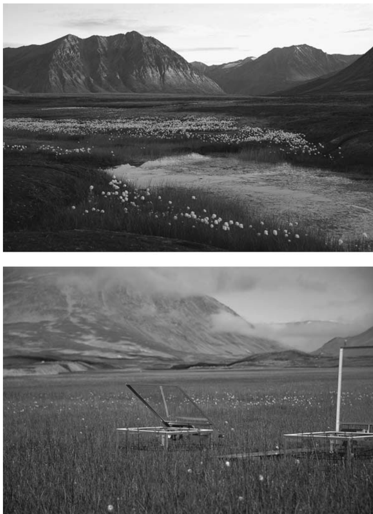
PLATE 1. (Top) Dense cover of Eriophorum spp. filling in a thermokarst erosion pond and (bottom) automatic chambers monitoring \text{CO}_2 and \text{CH}_4 exchanges in a tundra fen. Both photos were taken in Zackenberg Valley, northeast Greenland, a hotspot for both \text{CO}_2 exchange and \text{CH}_4 emissions. Photo credits: Torben R. Christensen.
