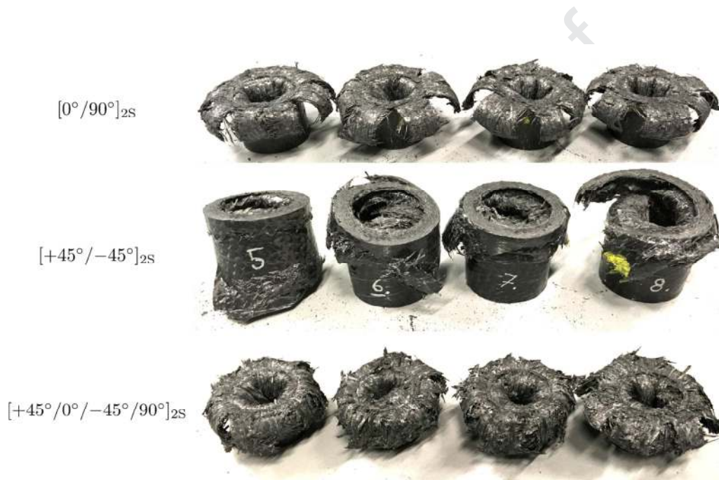
Figure 11 – Quasi-statically crushed tubular coupons for the three different layups.
