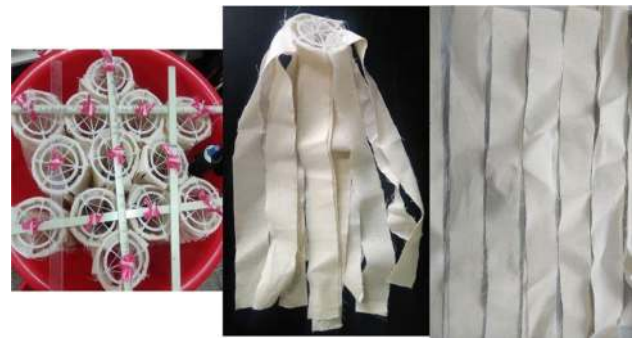
Fig. 2 Images of WCC strips used to make the biofilm carrier showing WCC strips (right), the biofilm carrier unit (middle) and those hanging in the reactor (left)
