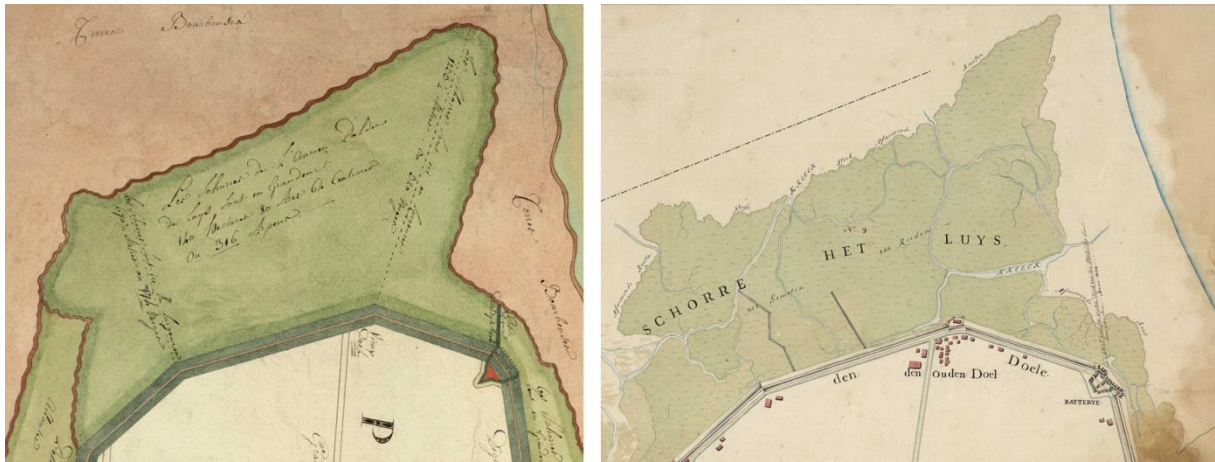
Figure 5. Two maps depicting the same part of the tidal marsh. Left a map from 1813 (ARA, Arenberg, 842) with an MPE of 103.68 meters, right a map from 1816 (ARA, Kaarten & Plans II, 8554) with an MPE of 32.54 meters. The map at the right with the lowest MPE was chosen for this part of the reconstruction of 1790.
