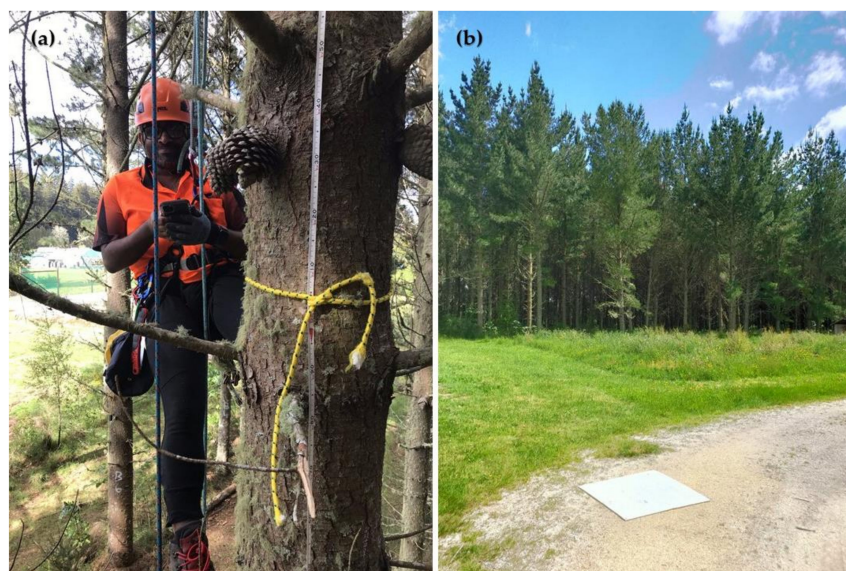
Figure 3. Images from the data capture showing (a) measurements being recorded to a mobile application during crown mapping and (b) a target deployed to the site as a ground control point.
