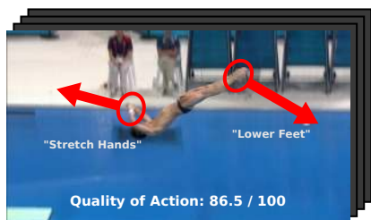
Fig. 1. We introduce a learning framework for assessing the quality of human actions from videos. Since we estimate a model for what constitutes a high quality action, our method can also provide feedback on how people can improve their actions, visualized with the red arrows.
