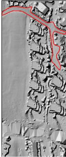
Figure 7. The red line polygon represents a road area selected based on visual analysis of the UAV orthophoto in order to quantitatively compare elevation, slope, and aspect of the two DEMs without the influence of objects such as vegetation, cars, or other features that are known to differ categorically between the two DEMs.
