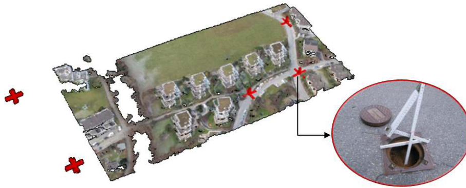
Figure 3. Left: locations of the georeferencing points used in the study (red crosses). While the left-most points are outside of the area of study, they were covered by UAV images. Right: measurement of vertical distance between GCP access cover and actual GCP point.
