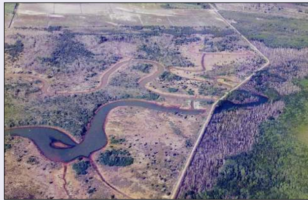
Figure 3. Trinity Inlet, Cairns, Queensland, Australia. The levee wall used to impound the wetlands is on the right. Degradation of vegetation is evident on both sides of the levee wall. Acid was released, soil C org was remineralized, and there was a 1.3 m loss in soil elevation (Hicks et al. 2003).
