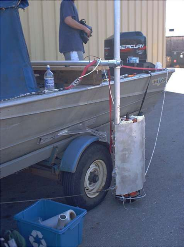
Fig. 1. RDI BBADCP boat-mounted for current transects in high flows.
