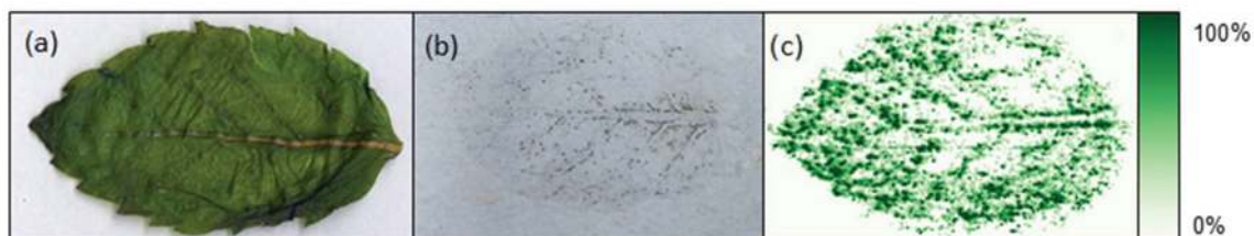
Figure 2. The optical images of (a) the peppermint leaf; (b) the resulting imprinting; and (c) the DESI image generated for the anion of m/z 299.05625 (deprotonated chrysoeriol (7)).
