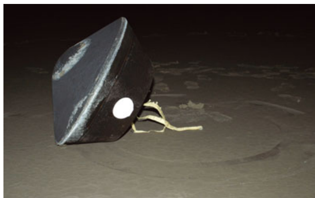
Fig. 16. The SRC as it was found upon recovery at the UTTR. The marks on the heatshield resulting from the initial impact on the SRC nose and one of the subsequent impacts on the edge of the SRC can clearly be seen in this picture. Two additional marks not visible in this picture, one on the rim of the heatshield and one on the edge of the backshell, were also apparent. The circle the SRC rolled in before coming to a stop is clearly apparent in the surrounding mud; the slight discoloration is due to small portions of the SRC’s thermal ablation materials that adhered to the mud as it rolled.
