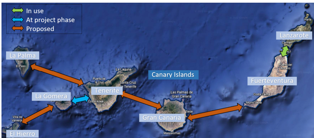
Figure 6. Proposed grid interconnection between the different islands of the Canary Archipelago.
