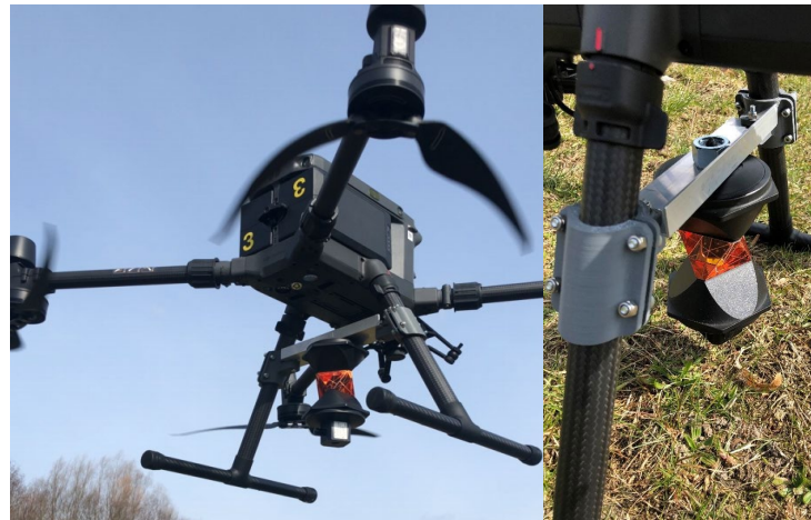
Figure 2. DJI MATRICE 300 RTK with Leica GRZ122 360° prism reflector.
