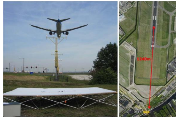
Figure 3: Experimental set-up located 1240 m to the South of the threshold of the Aalsmeerbaan (36R) Schiphol airport runway.
