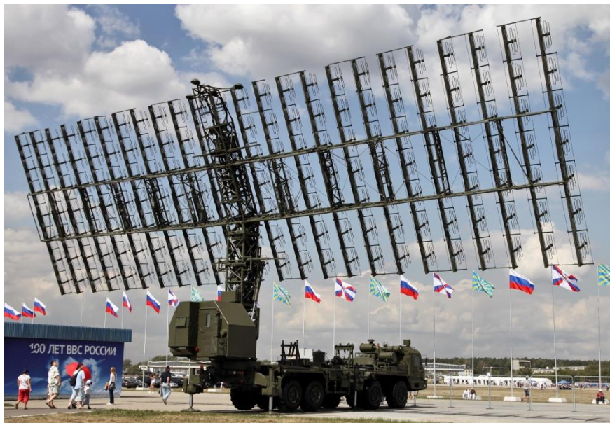
Figure 4. An acquisition radar operating on low carrier frequencies, designated 55Zh6M Nebo-M. ©Vitaly V. Kuzmin
