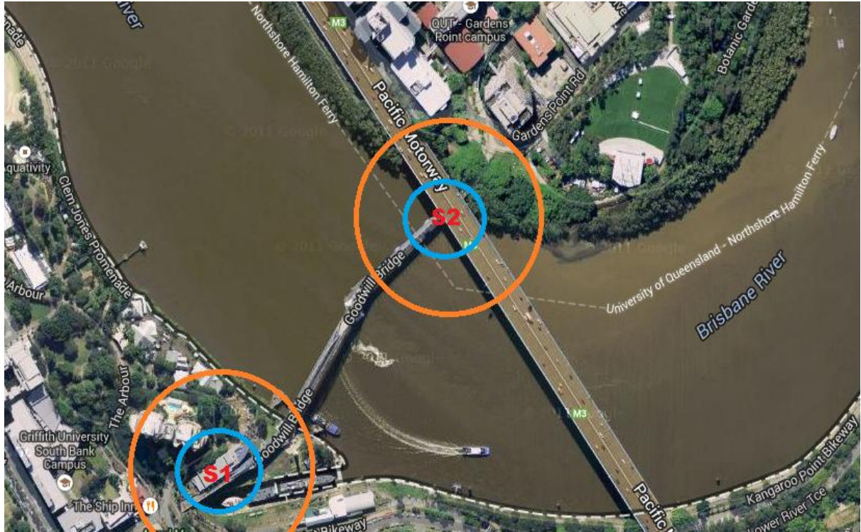
Fig. 3. Spatial map of study area. S1 and S2 show the location of scanning points. The detection range of 2dBi and 16dBi antennas are shown in blue and orange circles, respectively.
