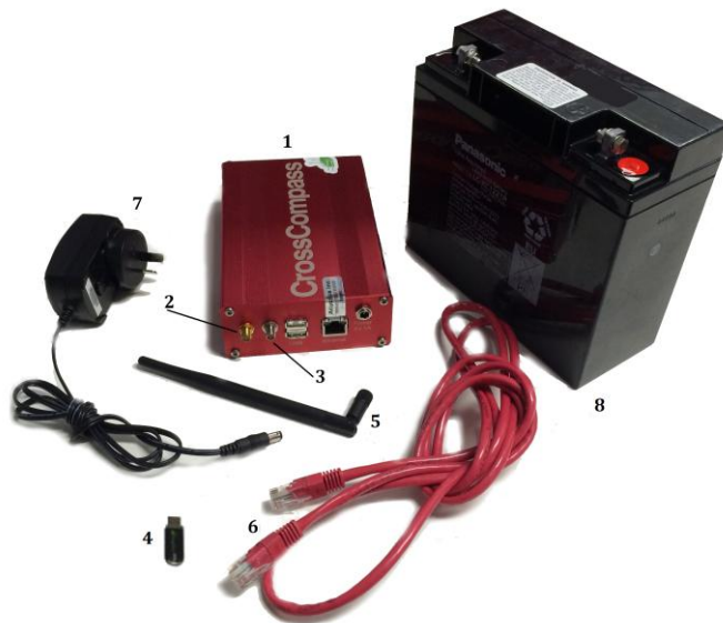
Fig. 1. Wi-Fi and Bluetooth MAC address scanning hardware used for data collection: computational unit (1), Wi-Fi (2) and Bluetooth (3) antenna connector, USB storage (4), omni-directional antenna (5), LAN cable (6) for data connection to PC, 240 v AC to 5 v DC power convertor (6) and rechargeable 14 v acid batter.
