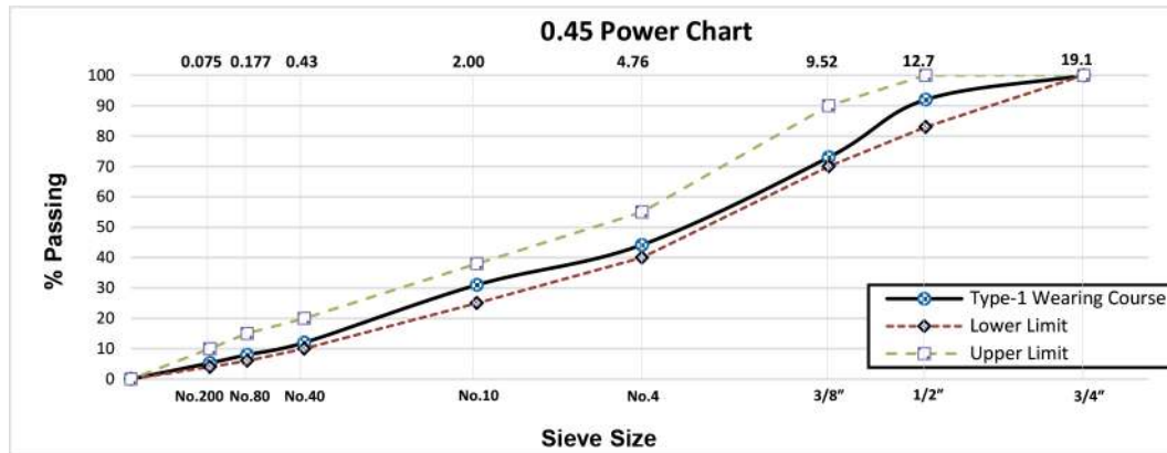
Fig. 2 Limestone 0.45 power gradation chart for the type-1 wearing course
