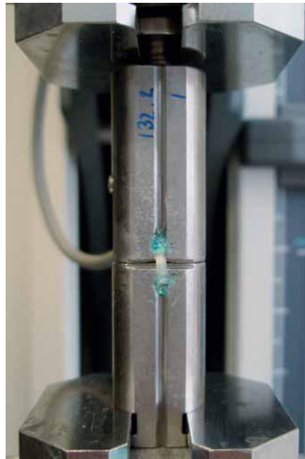
Fig. (3). The ends of a test specimen attached for tensile bond strength test.
