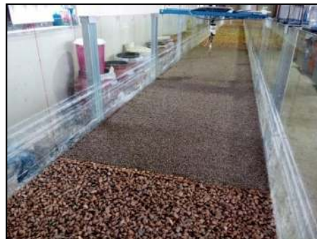
Figure 4. A view of the sand-bed section with coarse particles upstream and downstream.
