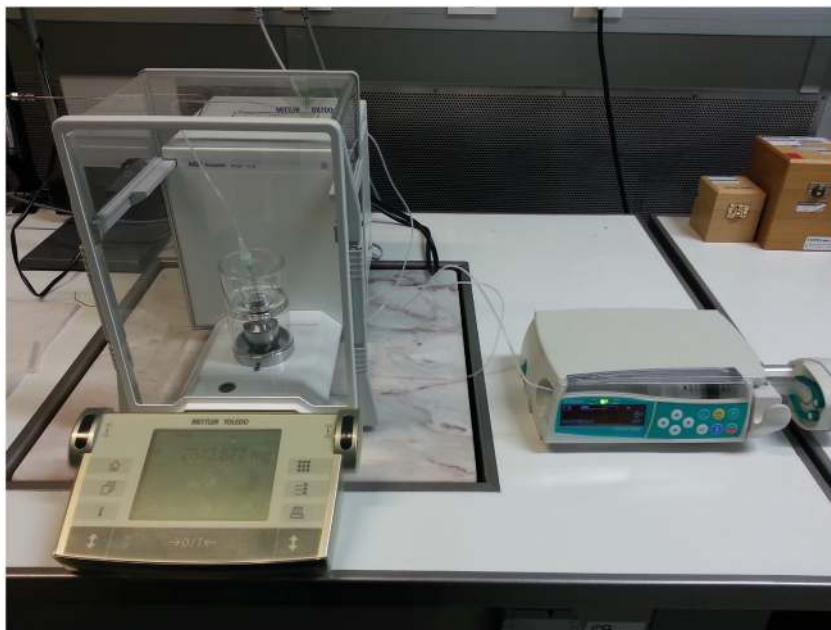
Figure 1: IPQ set-up for syringe pump calibration by gravimetric method.
