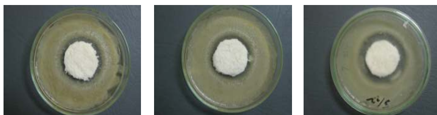
Figure 5. Zone of inhibition after 10 washing cycles of samples A-10, N-10 and HCAN-10.
