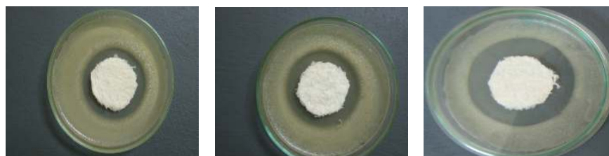
Figure 1. Zone of inhibition against E. coli of samples A-10, N-10 and HCAN-10
