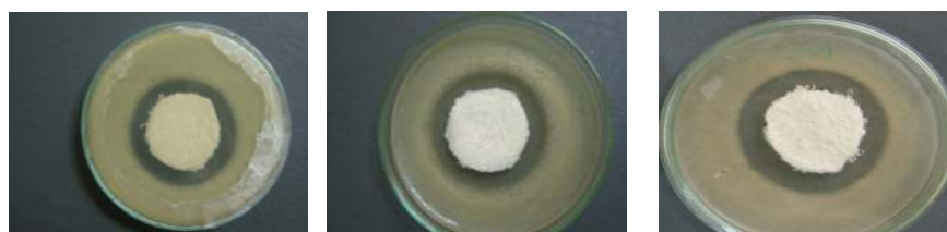
Figure 2. Zone of inhibition against S. aureus of samples A-10, N-10 and HCAN-10
