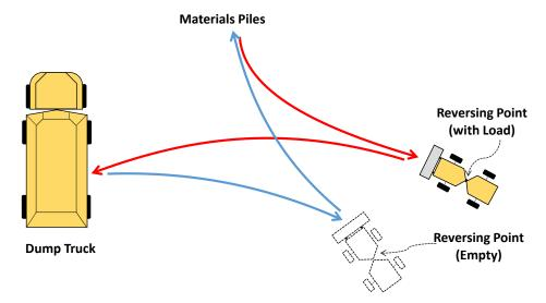
**Figure 6.** Schematic of an operational cycle of a wheel loader. The curved arrows are the trajectory for a wheel loader to complete a loading task.
