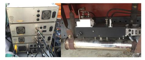
**Figure 2.** PEMS installed in dump trucks. The left is the gas analyzer units for measuring pollutants in the diluted exhaust; the right shows the sampling probes on the tailpipe with an exhaust mass flow meter.
