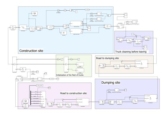
Figure A1. The SimEvents model for the earthwork project.
