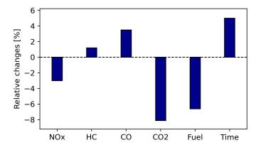
Figure 11. Relative changes in terms of emissions and fuel consumption.
