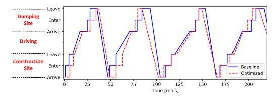
Figure 10. Timetable for 3.5 h of one DFL180 truck before and after the optimization.
