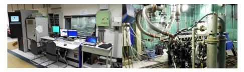
Figure 5. In-lab test: the test bench control platform (left) and the engine measurement system (right).
