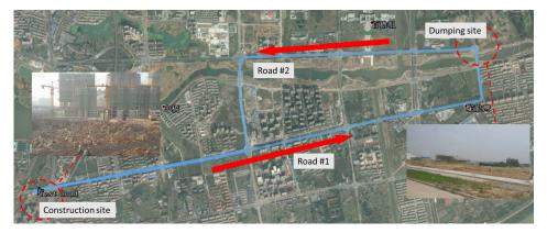
**Figure 3.** Hauling-and-returning routes (blue lines) of dump trucks for earthmoving. The Chinese letters on the map refer to the names of local places.
