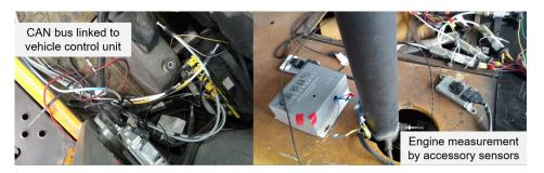
Figure 4. The vehicle data acquisition system and engine accessory sensors used in wheel loaders.
