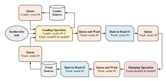
Figure 8. DES flowchart of the earthwork project.
