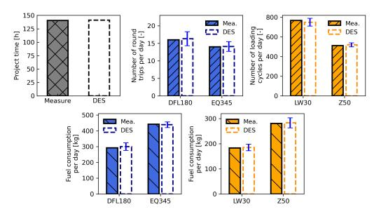
**Figure 9.** DES model validations against the real-world measurement. Error bars above DES bars represent the variation among simulation results.
