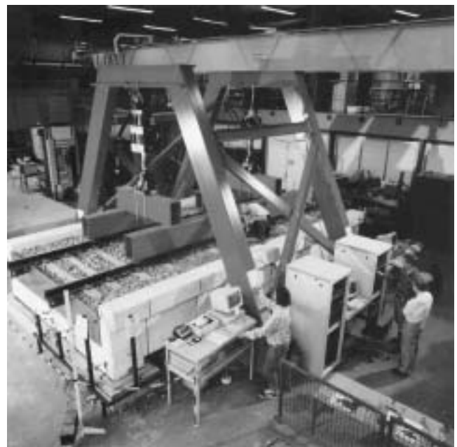
Figure 2. Concrete trough bridge with a span length of 7m being loaded in fatigue to assess its capacity to carry higher axle loads.
