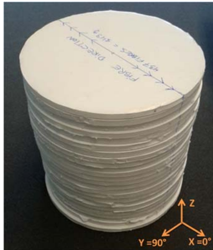
Figure 7. Cardboard specimen with aligned fibres
