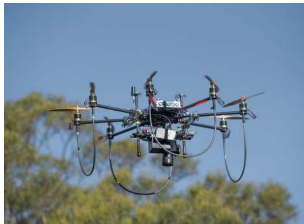
Figure 1. The small-UAV platform used to collect both airborne RGB photography and laser scanning data.
