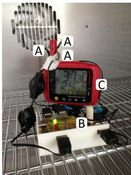
Figure 1. SHT21S sensors (A) connected to the Seeduino Datalogger (B) and placed close to the sensing tip of the Amprobe TR300 (C) in the oven.
